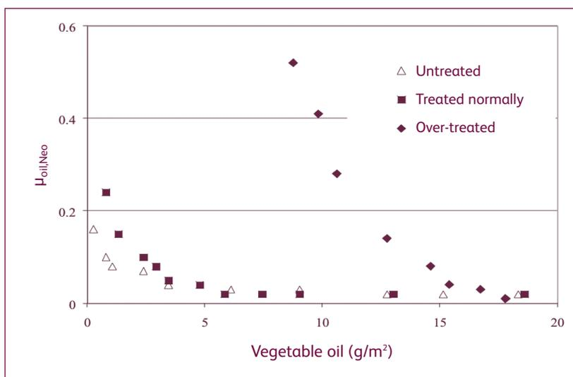
**Figure 8.0** Brungraber Mark II friction of a Neolite slider on oily glazed ceramic tiles. Untreated and clean tiles (Δ), tiles treated normally with the hydrofluoric acid solution (■) and tiles over-treated with the hydrofluoric acid solution (◆).
