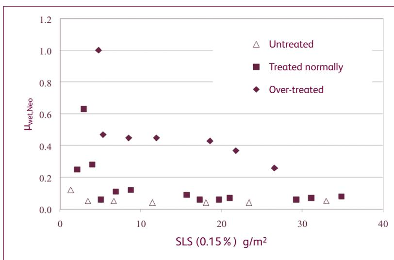
**Figure 7.0** Brungraber Mark II friction of a Neolite slider on wet glazed ceramic tiles. Untreated and clean tiles (Δ), tiles treated normally with the hydrofluoric acid solution (■) and tiles over-treated with the hydrofluoric acid solution (◆).
