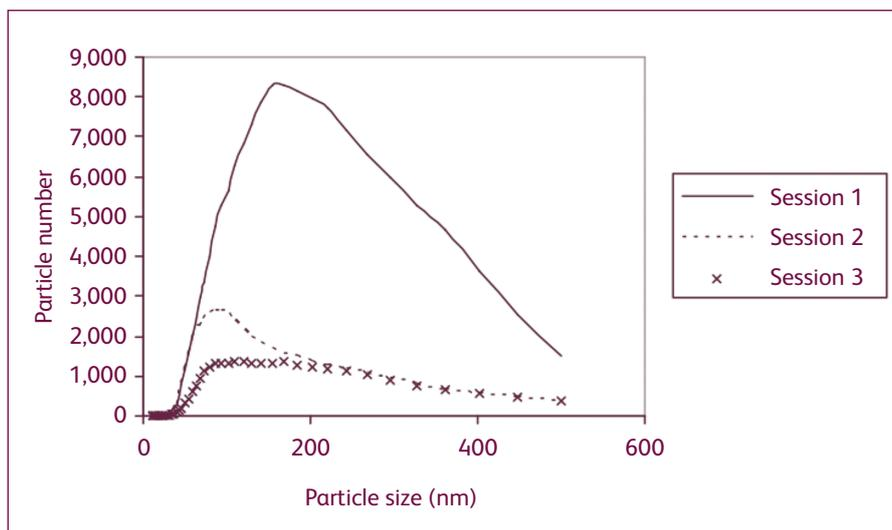
**Figure 4.0** Median particle number across the 10-500nm range measured during the three 30 minute smoking sessions.
